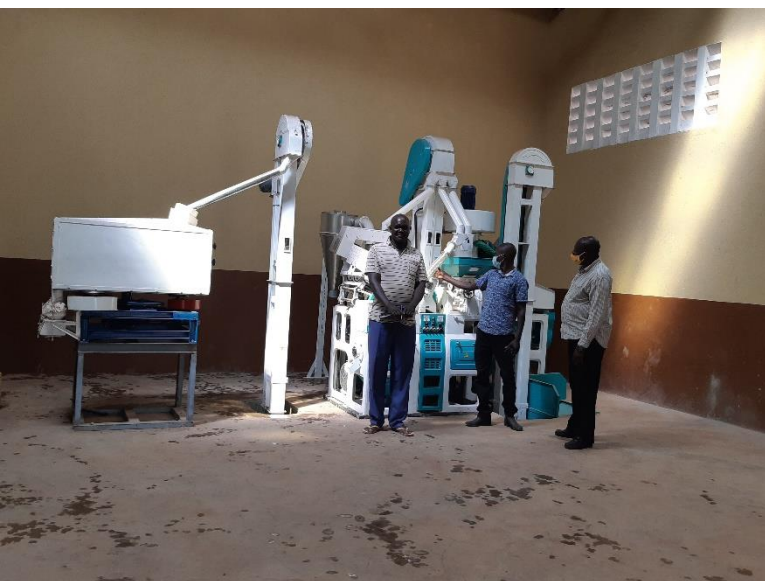
Installed rice huller at Amuru Tek Livestock Cooperative Miller
