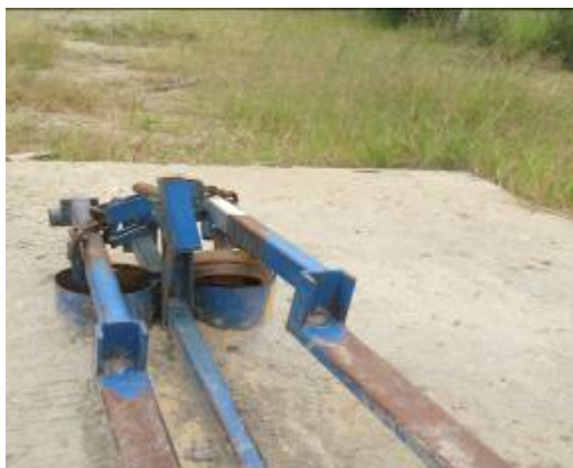
Photos 1&12: A broken down and unmaintained Triddle pump at Obwengerero Valley Tank, to the right is an empty cattle trough (Photo taken on 27/06/2011)
