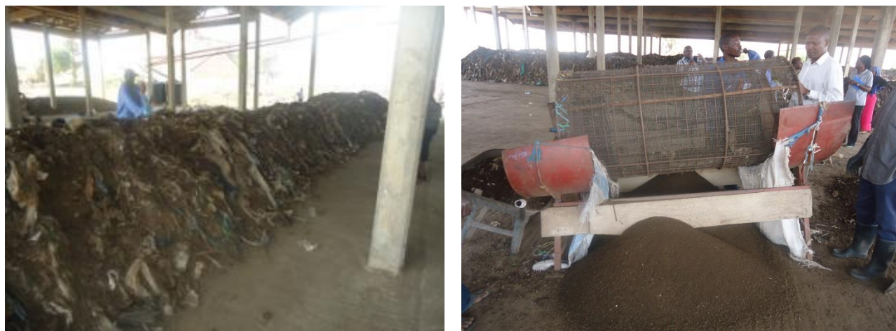
L-R: Windrow; Sieved compost at a CDM composting site in Mbale Municipality, Mbale District
