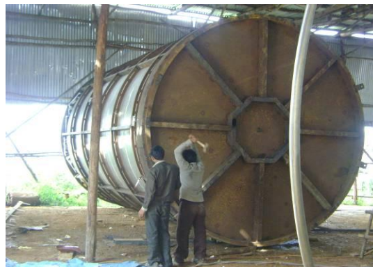
Left: Installations at the milk processing factory in Mbarara Right: Boiler being fabricated onsite.
