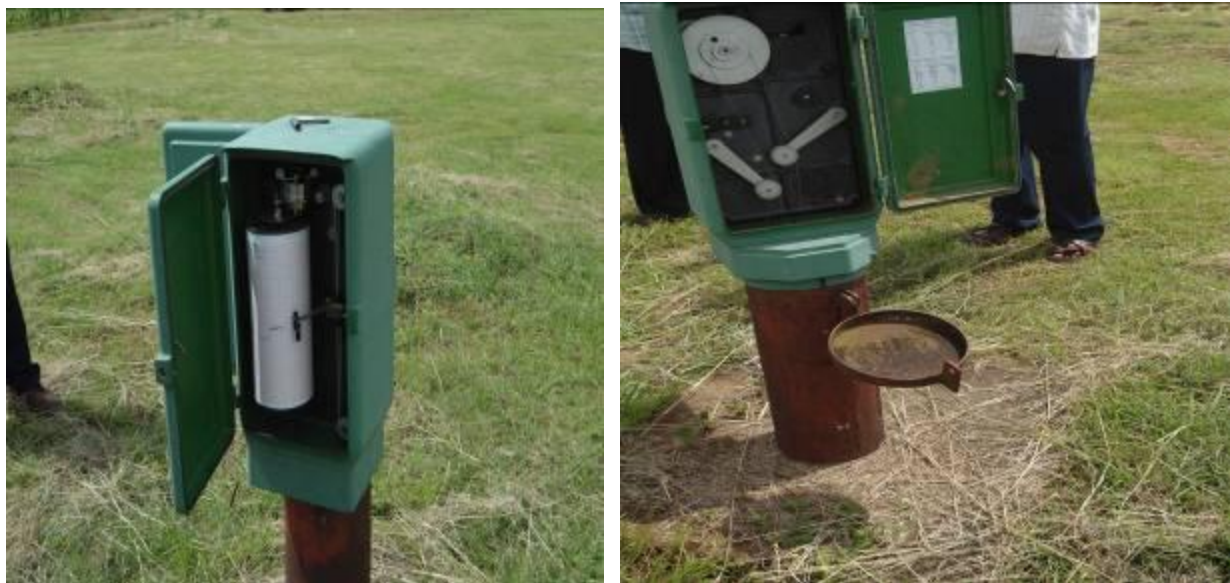
Photos 13&14: Ground Water Monitoring Station at Entebbe; To the left is the Guage Reader side that automatically plots the water levels the R16 automatic water level recorder and Water level meter (to the right) detect the underground water level movements.
