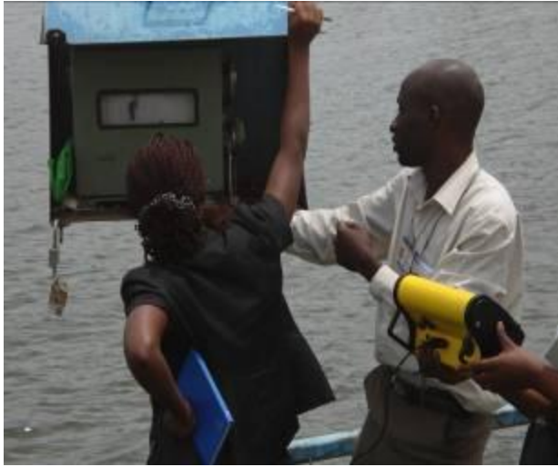
Photos 11&12: To the left Staff of SWRM showing the monitoring team how the Vota (yellow) is used to take readings from the Gauge Reader for data on surface water levels. To the right is an Acoustic Dopra Profiler measuring surface water levels.
