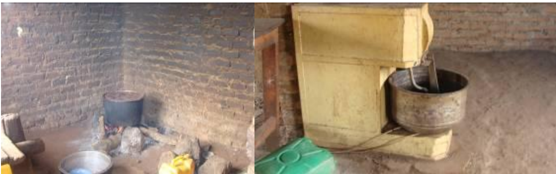
Three stone stove and electric dough mixture, all non-energy efficient cooking equipment used by the school.
